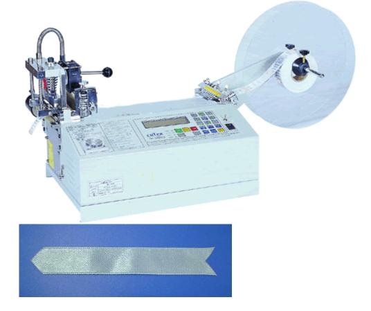
Model No. TBC-50H Cutting Knife HOT Maximum Cutting Width 30mm Range Of Cutting Length 15mm~300metres Cutting Quantity/Minute 120cut~140 cuts Packing Size 63×48×45cm(20.5/24.4kg) Application RIBBON TAPE, SMALL WEBBING, CAMERA LACE ETC. Cut-length is accurate owing to a stepping motor. Accuracy Because the hot knife melts the end of tape, cutting is sealed neatly Cutting type without fraying. Automatic operation It works automatically only by setting length and quantity.
